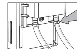
Decide which reservoir is correct for your installation. Ensure you have placed float magnet facing upwards and ensure 15cm x 6mm I/D breather tube is fitted to reservoir lid. Connect the water reservoir to the water drain of evaporator and ensure the top of the breather tube is above the max water level in the drip tray. Or if using other reservoir place and fix into condensate tray. Ensure reservoir is mounted horizontally.
